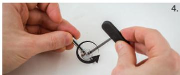
4. Disassemble two PatchWorks® Solderless 2-piece Plugs using the supplied PatchWorks TX8 wrench.
