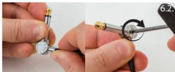
Assembling an angled **PatchWorks®** Solderless Plug:
