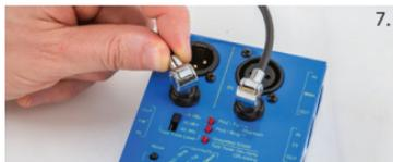
Repeat the above steps and complete the second plug of your new **PatchWorks®** Solderless Patch Cable. Use a cable tester to check the conductivity of your patch cables before using them.
