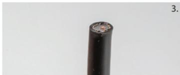
3. Take care that the cut is smooth and straight, to ensure good connection of the inner signal core and outer shield to the plugs as well as avoid shorts.
