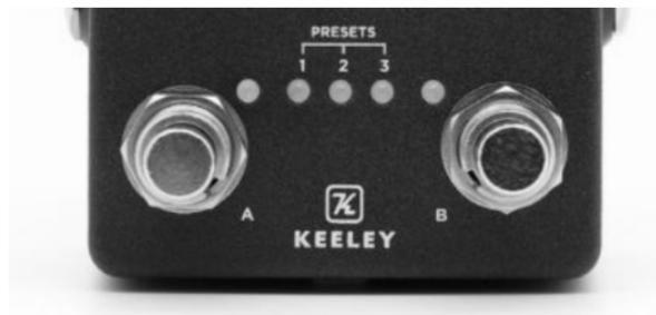
**SIDE A / B** - Tap the A or B footswitch to activate each side of the HALO. Tap the alternate footswitch to use the alternate sound stored in each Preset Bank.
