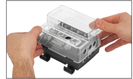
**IMPORTANT NOTE:** For mounting PedalSafe® Type E onto BOSS compact pedals, you must first detach the battery cover/footswitch plate by removing the screws before being able to pull the PedalSafe® shell over the pedal. Afterwards, reattach the battery cover/footswitch plate again.
