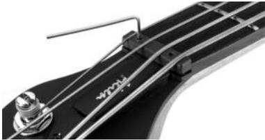
Use a 1.5 mm Allen wrench to adjust the string's height at the nut.
