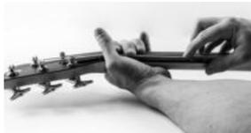
Check the distance between the first fret and the string. It shouldn't read more than 0.3 mm /0.01", which equals the thickness of a business card.
