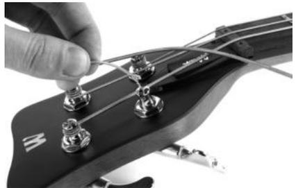
The tuner's post has a slot with a hole in the center. Put the string in that hole before you start winding. This system avoids the string poking out to the side of the tuner and stabilizes the winding and thus the tuning overall.
