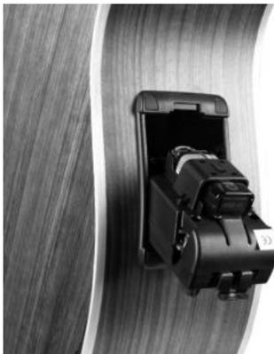
The battery and electronics compartment can be easily opened with your fingernail. Push the battery in until it locks in place.
