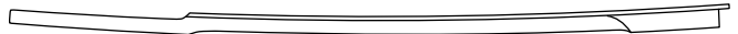
Loose truss rod with up-bow in the neck (concave), high string action.
