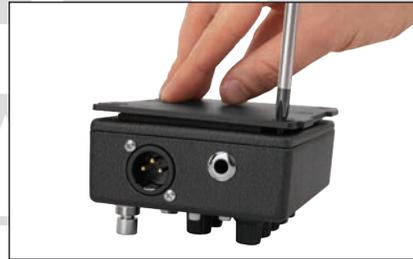
**IMPORTANT NOTE:** For mounting PedalSafe® Type E onto BOSS compact pedals, you must first detach the battery cover/footswitch plate by removing the screws before being able to pull the PedalSafe® shell over the pedal. Afterwards, reattach the battery cover/footswitch plate again.
