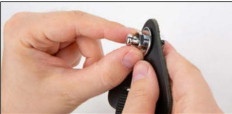
Screw the nut tightly onto the thread. To be on the safe side, tighten the nut with a suitable wrench.
