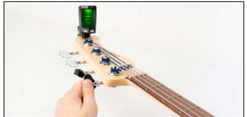
*To make sure the string is firmly seated and is properly wrapped around the post, you should lightly pull on the strings when you tune. Grab the middle of the string and pull it up to tighten the winding. Then re-tune.*
